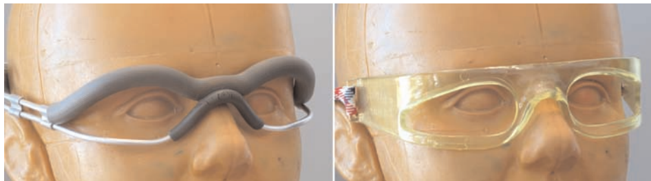
Figure 16. The original (ineffective) eye guards for handball, squash, and racquetball
