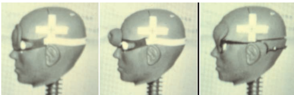
Figure 17. Racquetball eyeguard testing for ASTM F803 (1983)
